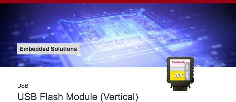
Transcend's USB Flash modules are convenient, easy to implement solutions for expanding the memory capacity of industrial computers. These compact storage devices consume a minimal amount of power and feature a mechanical write protection switch. Due to their minimalist dimensions, these USB modules are suitable for use in small embedded systems.
