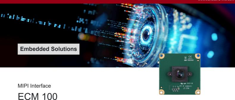
Designed for embedded systems and intelligent applications, Transcend's industrial-grade ECM100 Embedded Camera Module is equipped with the high-sensitivity Galaxycore 2093 CMOS sensor. It delivers 2MP resolution and a 130° field of view, producing sharp, low-noise images even in low-light environments. Supporting the MIPI CSI-2 interface, the ECM100 can be seamlessly integrated into various embedded platforms, including AI edge computing, industrial inspection, and robotic systems.
