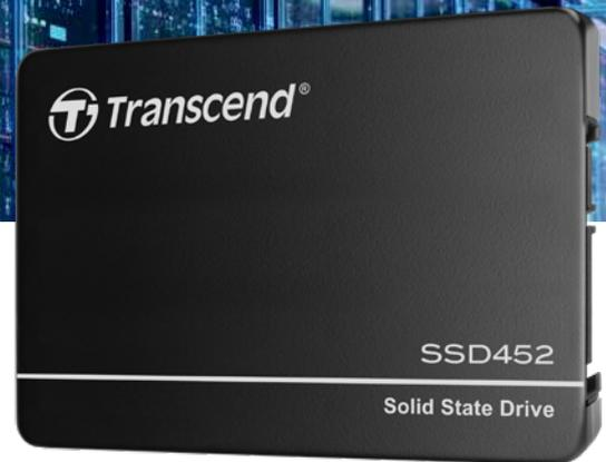
Transcend's SSD452K features the SATA III 6Gb/s interface and state-of-the-art BiCS4 technology, which allows 96 layers of 3D NAND flash chips to be vertically stacked. Compared to BiCS3 NAND at 64 layers, this density breakthrough greatly improves storage efficiency. The SSD452K is built with DRAM cache for fast access, and is fully tested in-house to guarantee reliability in mission-critical applications, boasting an endurance rating of 3K Program/Erase cycles.
